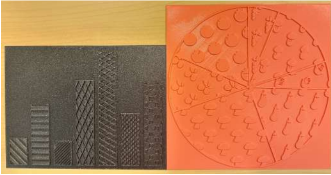
Fig. 7: Two 3D printed textured charts, one with geometric textures, and another with iconic textures.
